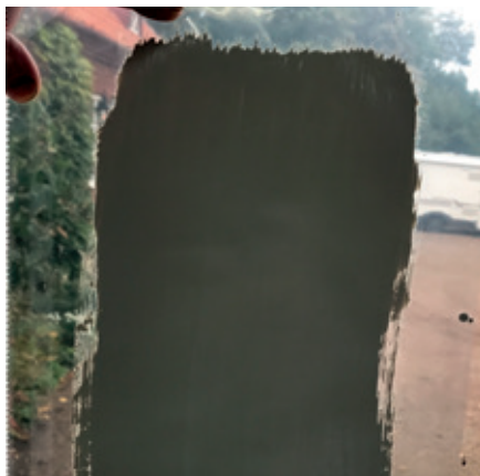
Each coat should provide full coverage. Approx. 100 microns per coat.
